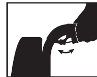
Figure 12. Manual Recline—Minimum and Maximum Recline Angles
