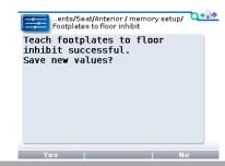
When the articulating foot platform is moved closer to the floor, the power base will go into drive lockout. This is to make sure while the footplates are closer to the ground, that the consumer can not drive their power chair, and potentially cause damage to their foot platform.
